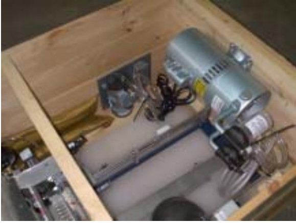
Air compressor is also secured to side of crate. Notice the wood brace across the middle of the crate
