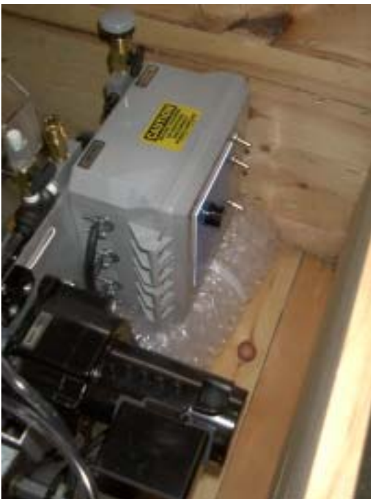
Padding to support the weight of the control box is important.
